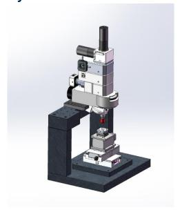
The MIC-PL(XXX) series is the nominal model of the micro-area laser excitation fluorescence spectroscopy measurement system, where XXX represents the wavelength. The imaging quality is comparable to a standard microscope.
